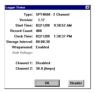
Displays operational information about the logger such as logger type, firmware revision, start time, record count, clock time, present reading for each channel, channel configuration, battery voltage, and whether Wraparound recording is enabled. This is a useful function for verifying that the logger is operating properly and communicating with the PC.
