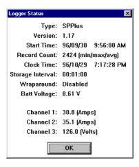
Displays operational information about the logger such as logger type, firmware revision, record count, clock time, present reading for each channel, channel configuration, battery voltage, and whether Wraparound recording is enabled. This is a useful function for verifying that the logger is operating properly and communicating with the PC.
