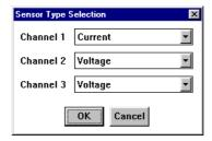
Pressing the Sensor button allows you to define what type of input each channel is to have. Presently, the *Silent Partner SPHD* supports voltage and current inputs.
