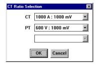
Pressing the Range button allows you to select from a list of preconfigured CT or PT ranges. Note that only one range can be set for each data type. For example, if you were recording two currents and one voltage, you would be able to select one range for current and one range for voltage.
