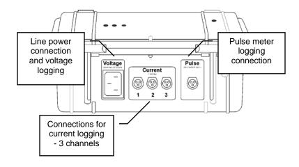
The connections to the logger are located on the side of the unit.
