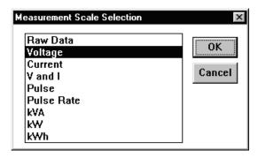
13. Select **kVA**, **kW** or **kWh** to display the power data. Note that total kWh data is displayed as bar graphs rather than line graphs.
