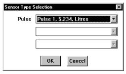
9. Open the **Pulse** drop-down list and select the appropriate sensor type. Then click **OK**.
