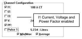
The number of Current channels you enable determines the Supply Types from which you can choose in the Ratio/Power Selection dialog box. Refer to **Displaying Power Data**.
