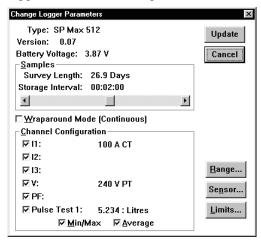
To adjust the Survey Length and Storage Interval move the slider.
