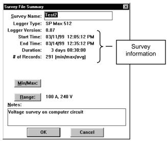
To display the minimum and maximum readings during the survey period for the display group you have selected, click the <u>Min/Max</u>: button. The minimum and maximum values are displayed in the format shown below. To close the Data Min/Max Values dialog box, click **OK**.
